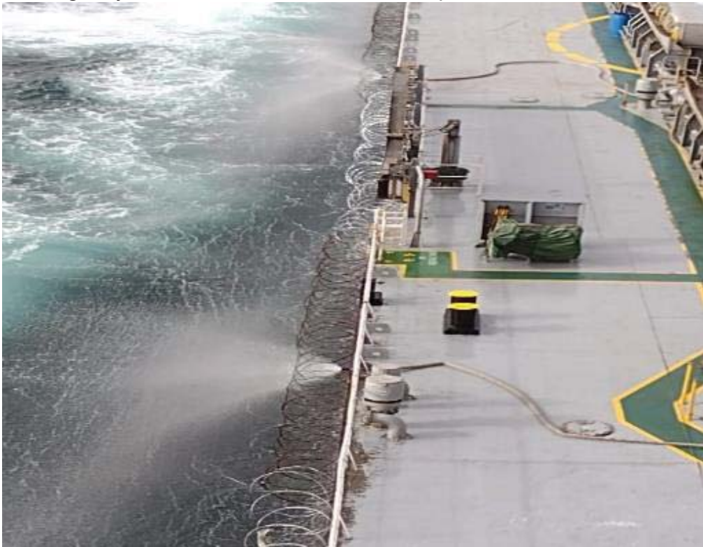
Contingency actions carried out. Fire hoses port & starboard were activated
